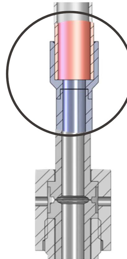
3 - 4 VCR water connections per target
