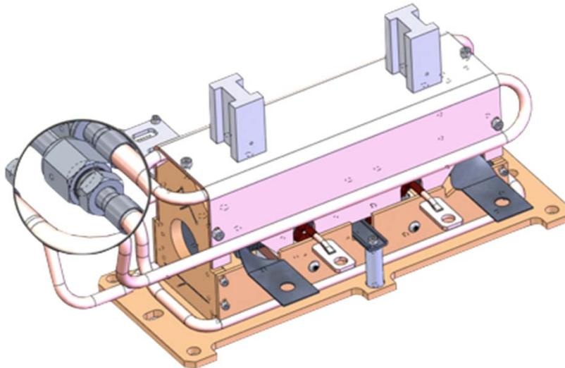
3 - 4 VCR water connections per target
