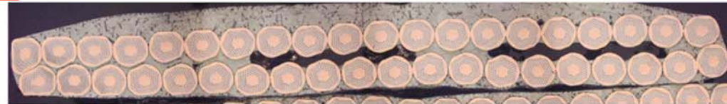
DS Dipole cable – 40 Strands (0.7 mm) Width = 14.7 ... 15.1 mm, Twist Pitch = 100 mm, 0.8° keystone
