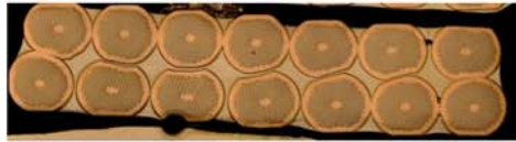
SMC Dipole cable – 14 strands (1.25 mm) and 18 Strands (1 mm), Width = 10 mm, Twist Pitch = 60 mm
