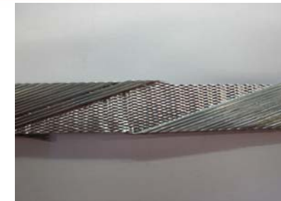
DS Dipole cable – 40 Strands (0.7 mm) Width = 14.7 ... 15.1 mm, Twist Pitch = 100 mm, 0.8° keystone
