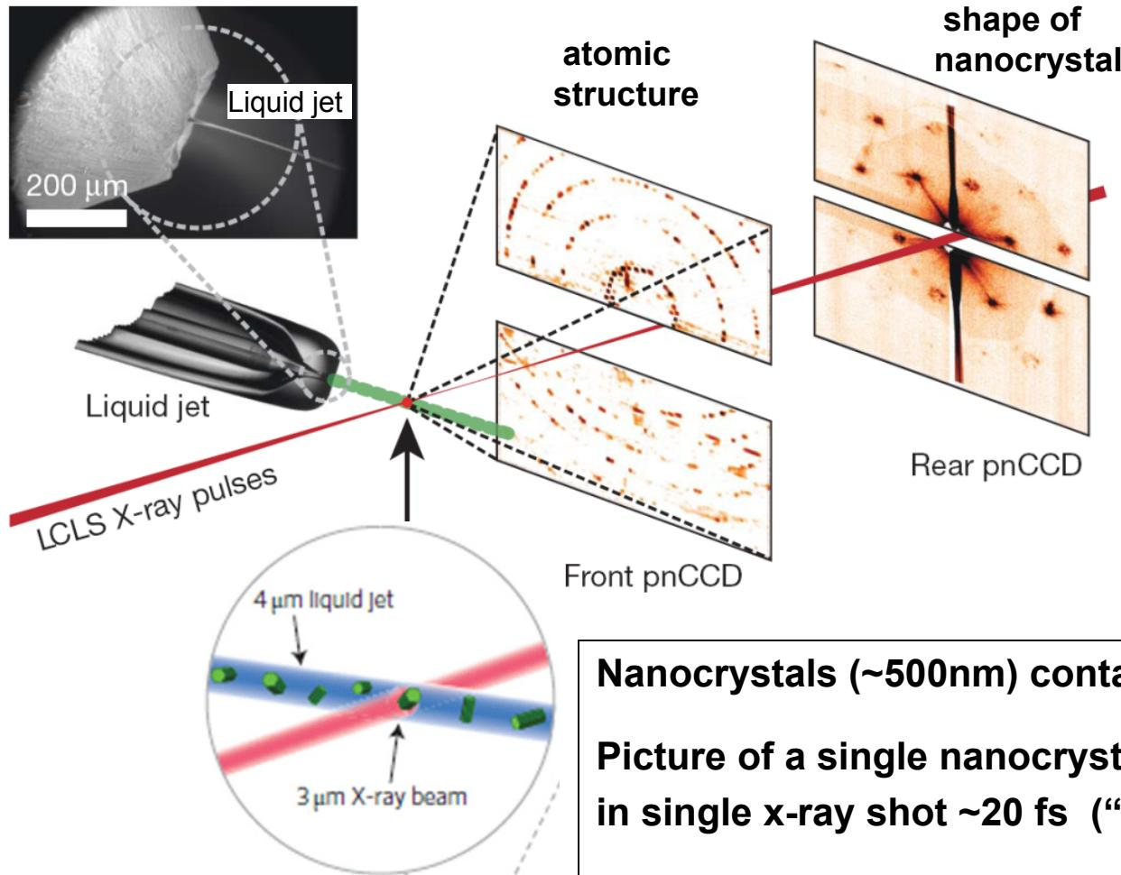
**Nanocrystals (~500nm) contained in water jet**
