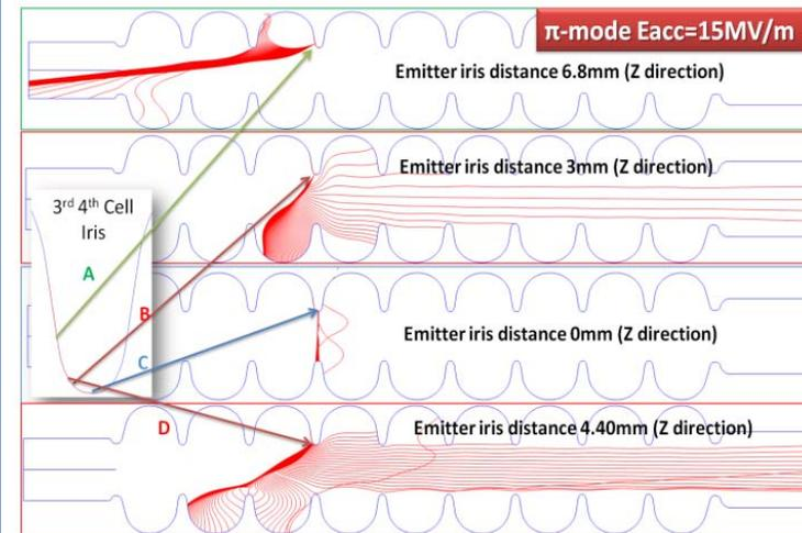
Trying to deeply understand phenomena of field emission by calculation, using Fishpact
