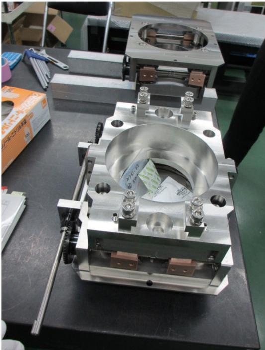
Frequency tuner: fabricated
