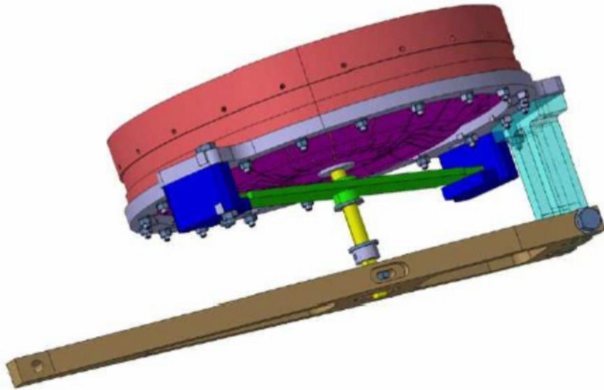
Pictorial view of the tuning plate with its actuator
