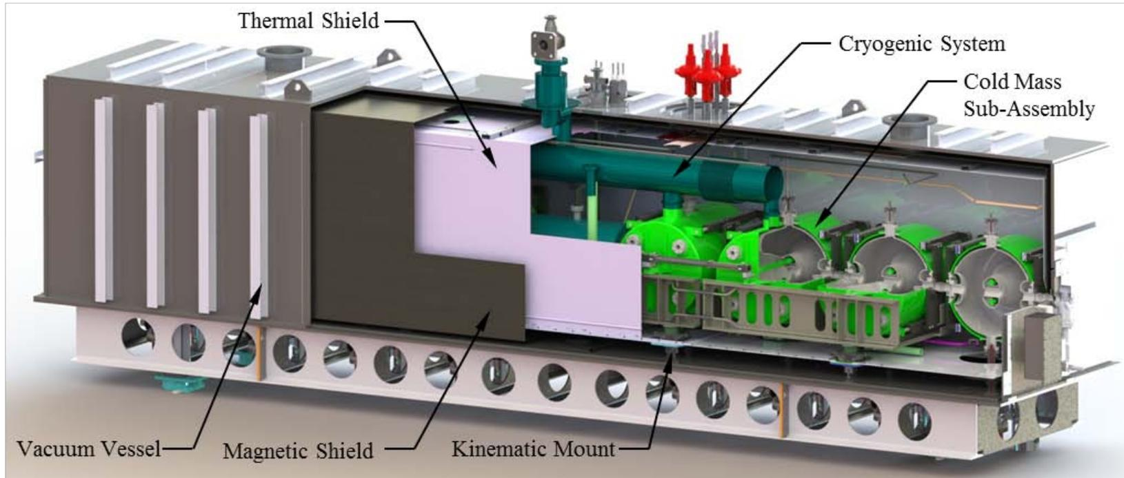
322 MHz,  $\beta = 0.53$  Cryomodule
