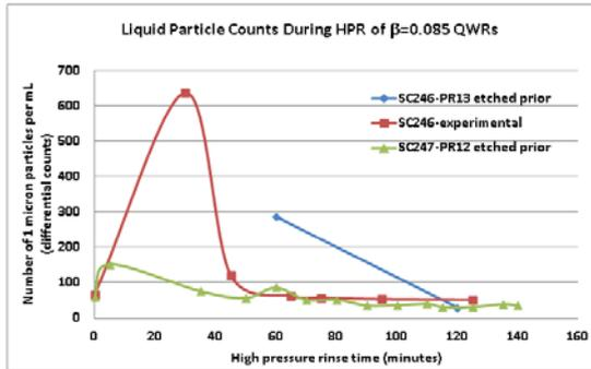
Liquid (left) and surface particle count for HPR water and resonator cleanliness monitoring
