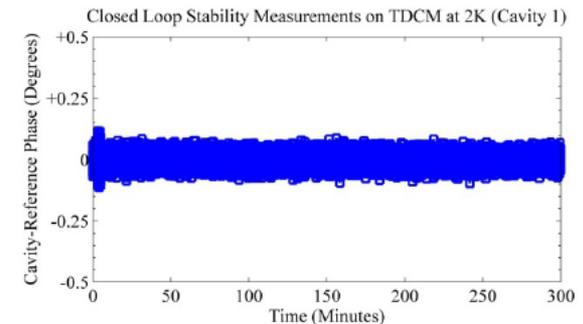
Phase and amplitude stability of HWR locked at low field at 2K
