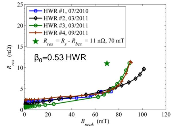
Residual surface resistance  $R_{res}$  vs.  $B_p$  measured in the FRIB prototypes at 2K
