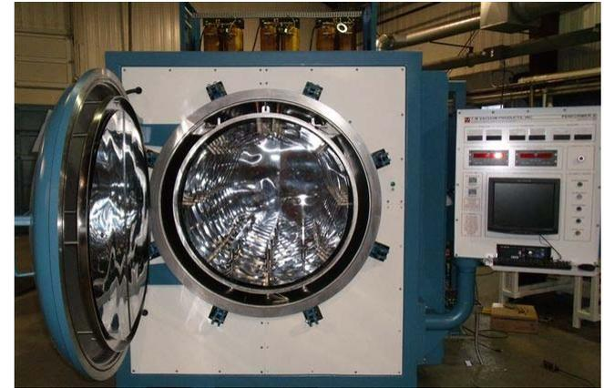
HV furnace for 600° C baking
