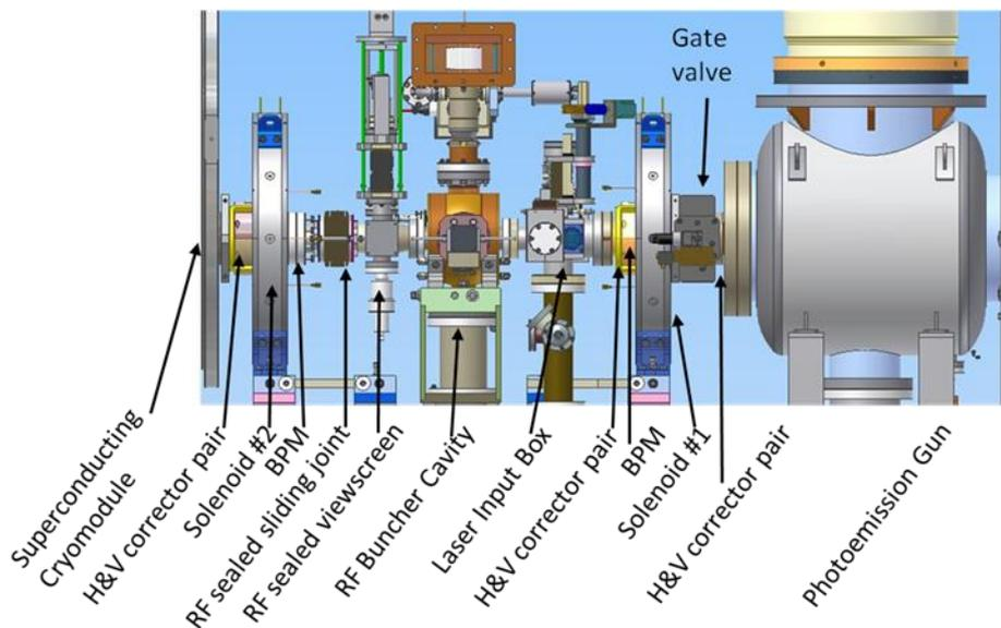
Aligning the magnetic and electrical centers of all elements to the beam axis is crucial for obtaining low emittance and minimizing aberrations.
