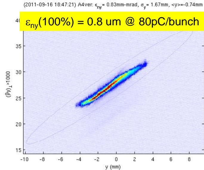
At 5 Mev, 80 pC we are within 40% of the simulated emittance and 80% above the thermal emittance of the cathode.
