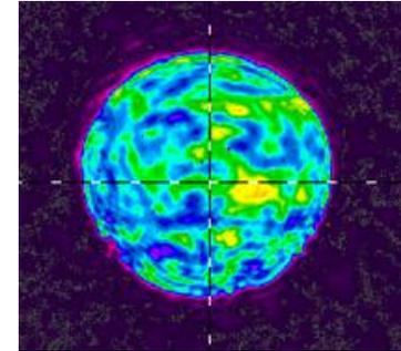
Our final laser mirror scattered ~50x more light compared to dielectric mirrors (which we cannot use). A new mirror with 2 nm-rms surface roughness was installed to fix the problem
