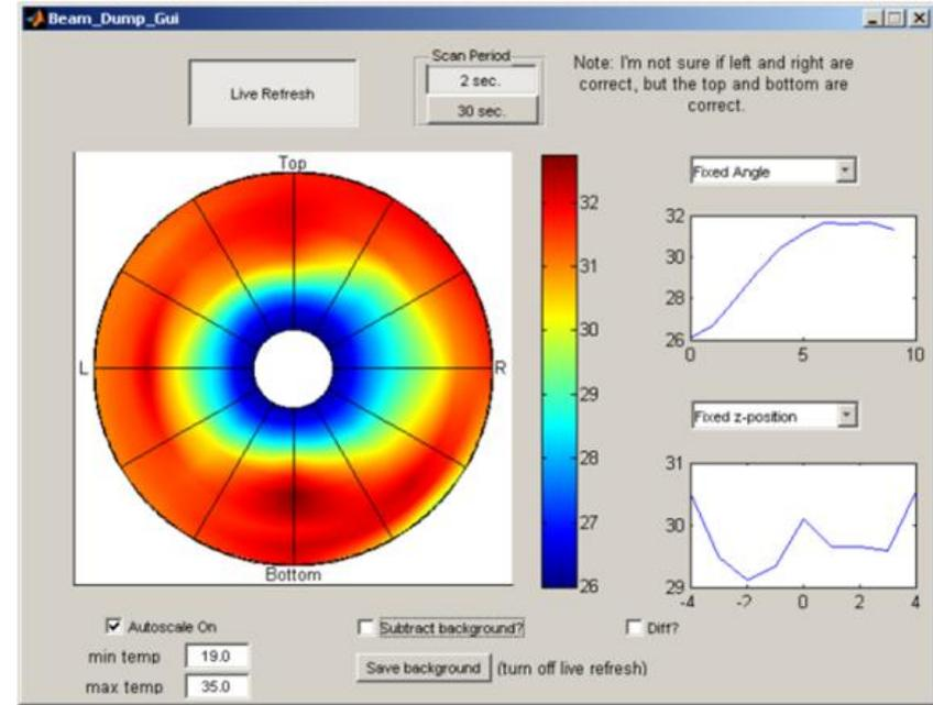
In this view, the water flows from the center (end of dump) to the outside (front of dump)
