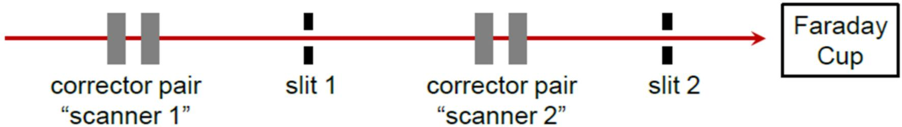
Leave the slits stationary and scan the beam across them. Can measure charge ranges from 0.1 pC up to 100 pC. Measurements take ~10 seconds.
