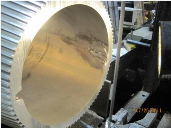
We burned a hole in the aluminum dump at 25 mA. This was due to the incorrect setup of the raster/defocusing system, and one shorted magnet.
