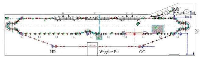
Figure 1: JLab IR and UV FELs in facility, showing SRF linac (top), IR recirculator (middle) and UV recirculator (bottom). The UV High Reflector vacuum vessel (HR), wiggler pit, and UV Out-Coupler (OC) locations are indicated.
