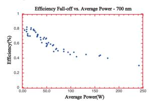
Figure 4: 700 nm lasing efficiency vs. power.
