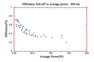
Figure 3: 400 nm lasing efficiency vs. power.
