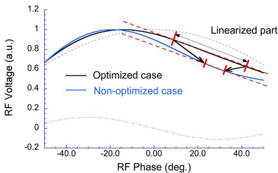
Figure 2: Schematic view of non-optimized linearization.
