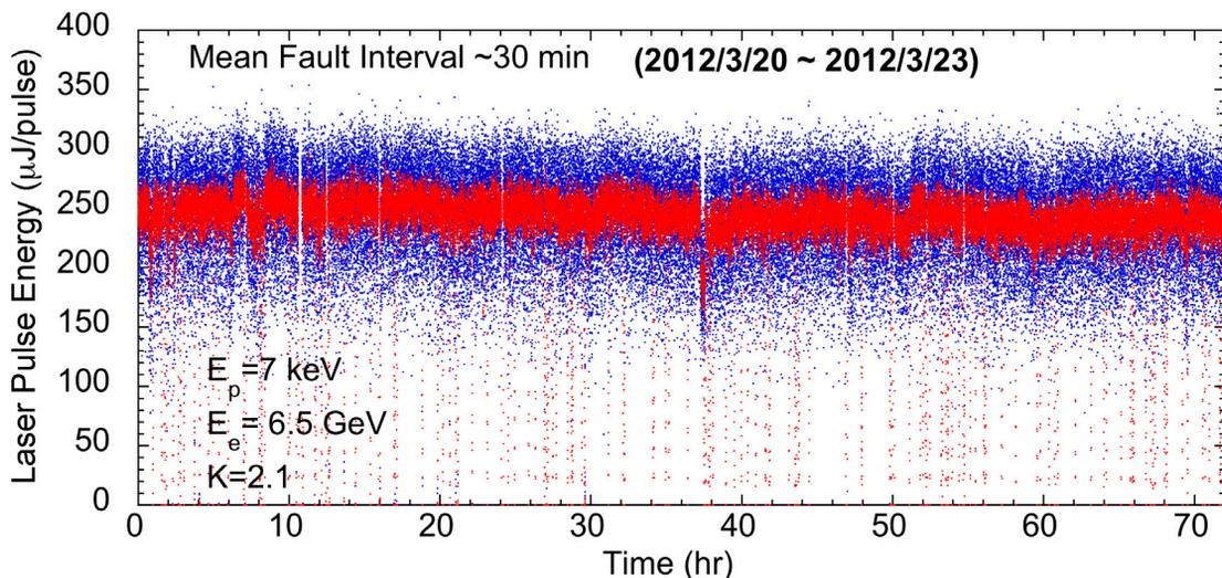
Figure 6: Intensity fluctuation and drift of SASE XFEL over 3 days. The blue and red points represent single shot pulse energy values and 10 shots moving averaged ones.
