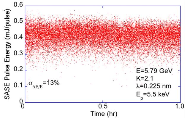
Figure 5: Intensity fluctuation of SASE XFEL over 1 hr.
