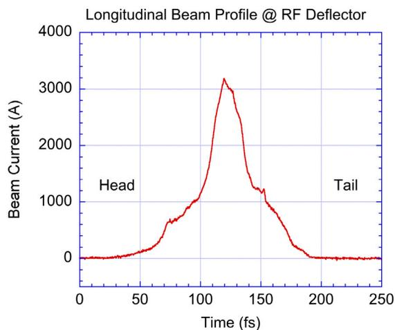
Figure 4: Typical electron beam temporal profile measured by RF deflector system after full bunch compression.
