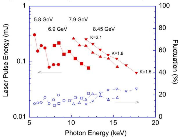
Figure 3: Dependences of pulse energy and intensity fluctuation on beam energy and a K-value. The symbols on each line for the constant operating energy show different K-values from 1.5 to 2.1.
