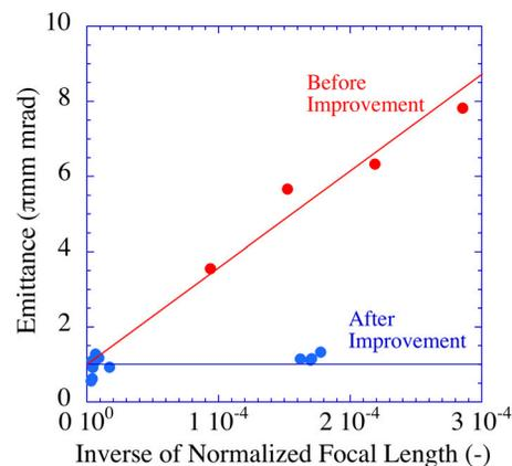
Figure 1: Correlation between an evaluated emittance value and a focal length of a Q-scan system at the exit of BC3 before and after the improvement.
