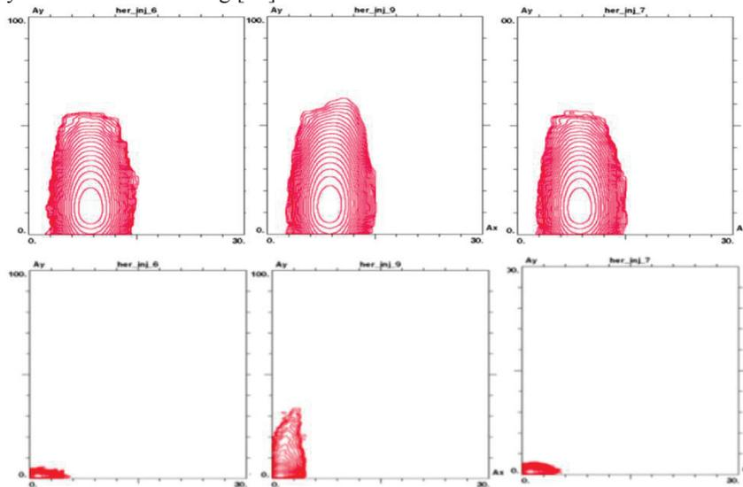
Figure 7: Effect of crab sextupoles on injected beam. Top: injected beam, bottom damped beam. Left: no bb interactions, center: bb interactions + crab sextupoles OFF, right: bb interactions + crab sextupoles ON.
