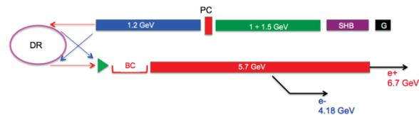
Figure 6: SuperB Injection system sketch.
