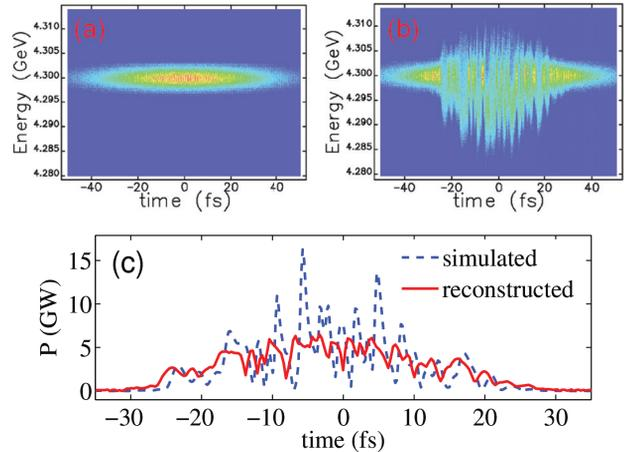
Figure 2: Beam longitudinal phase space with FEL off (a) and on (b); (c) X-ray power profile (provided by Y. Ding).
