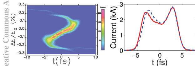
Figure 1: (Left) Longitudinal phase space for the under-compressed LCLS beam; (Right) True temporal profile (red) and predicted temporal profile (blue) from the longitudinal-to-transverse mapping technique (from Ref. [9]).
