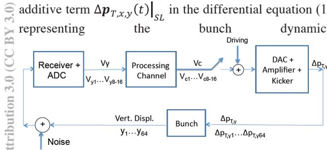
Figure 2: Block diagram of single-bunch feedback system
