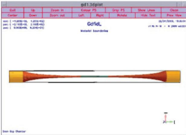
Figure 2: The vertical profile used in numerical simulation of an optimized nonlinear taper connecting regular APS chamber to an undulator chamber with an 8-mm vertical gap.
