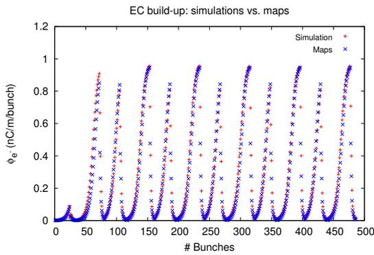
Figure 3: Comparison between the electron flux per bunch obtained with full simulations and applying map formalism considering a realistic pattern.
