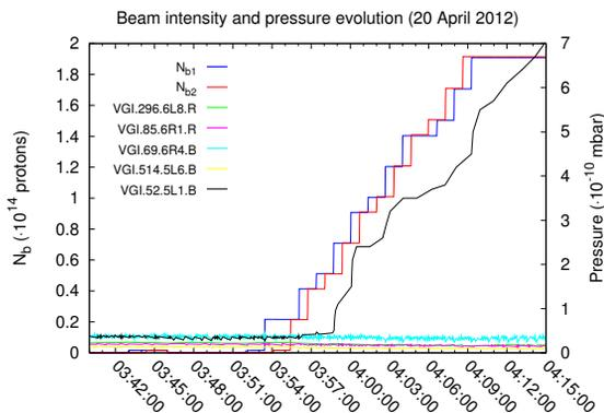
Figure 2: Pressure evolution during injection of physics fill on 20 April 2012. The five gauges shown are placed in different sectors, three corresponding to beam 1 and two to beam 2. The sector 5L1 was opened during the shutdown and exhibits pressure rise in the single-beam-pipe gauge VGI.52.5L1.B.
