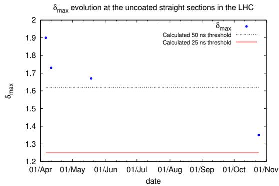
Figure 1: Estimated evolution in time (from April to October 2011) of  $\delta_{\max}$  in the uncoated straight sections of the LHC. The lowest value reachable with scrubbing corresponds to the 25 ns thresholds. The first injection with a 25 ns bunch spacing beam took place on 29 June 2011. The thresholds for 25 and 50 ns have been calculated for  $R = 0.3$  and  $N_b = 1.1 \cdot 10^{11}$  ppb
