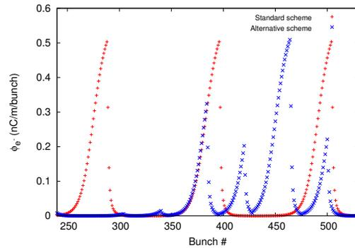
Figure 5: Comparison between a standard and an alternative filling scheme. The region shown is a fraction of an LHC turn of the length of the alternative pattern.
