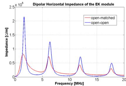
Figure 6: Driving horizontal impedance of the EK PSB kicker open terminated at both end (blue) and with one end matched and the other open terminated (red).
