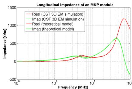
Figure 5: Comparison of the longitudinal impedance for an MKP-L module of CST 3D TD simulations (dashed lines) with the theoretical model (full lines).
