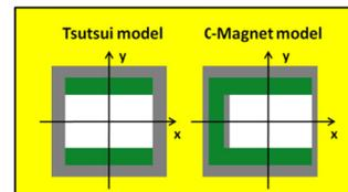
Figure 1: Geometric models for impedance calculation: ferrite in green, PEC in gray and vacuum in white.
