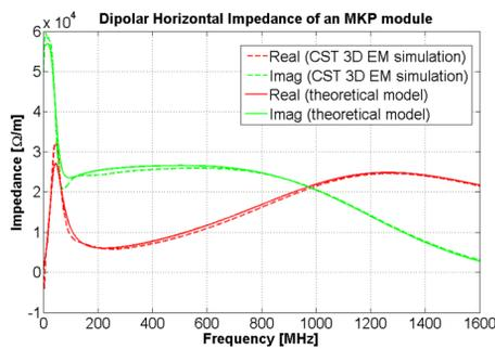
Figure 4: Comparison of the driving horizontal impedance for an MKP-L module of CST 3D TD simulations (dashed lines) with the theoretical model (full lines).
