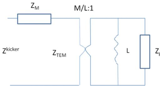
Figure 3: Circuit model of the kicker including cables.  $L$  is the inductance of the magnet circuit,  $Z_g$  the external impedance including cables,  $M$  the mutual inductance of the magnet.
