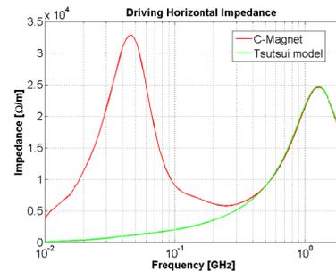
Figure 2: Simulations of the real part of the driving horizontal impedance for an MKP-L (SPS Injection kicker) module using different models.
