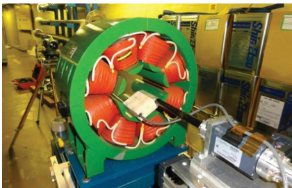
Figure 3: The octupole magnet and magnetic field measurement devices.
