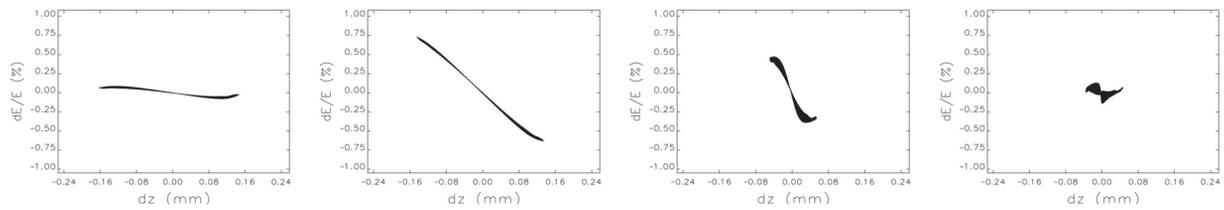
Figure 2: Longitudinal phase spaces ( $dz$  (mm),  $dE/E$ ) along the beamline; at  $z = 0.70$  m,  $1.05$  m,  $2.50$  m, and  $3.00$  m from left to right.
