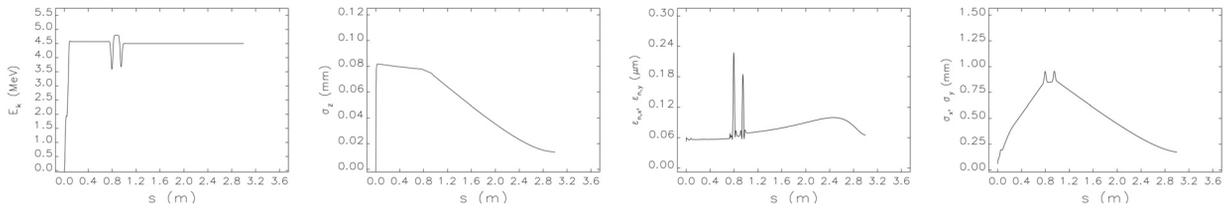
Figure 3: Optimized beam parameters along the beamline; kinetic energy, rms bunch length, normalized transverse emittance, and rms beam size from left to right.
