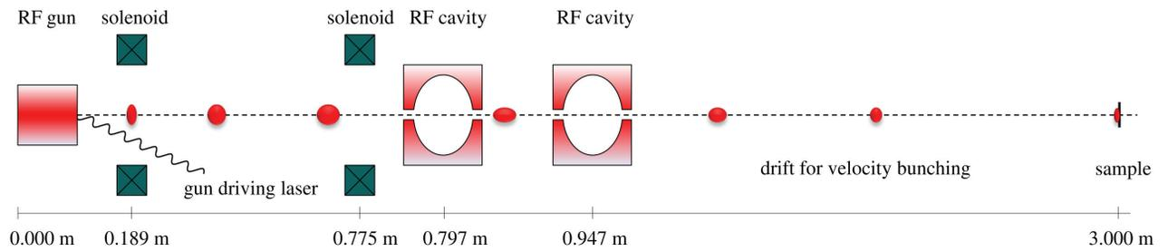
Figure 1: Layout of a 3 m long compact linac for an UED facility.
