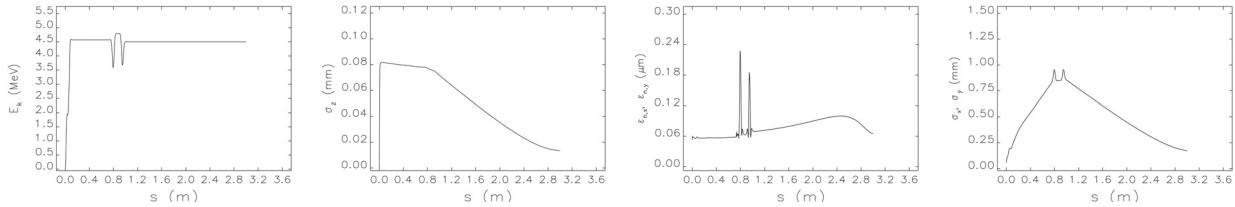
Figure 3: Optimized beam parameters along the beamline; kinetic energy, rms bunch length, normalized transverse emittance, and rms beam size from left to right.
