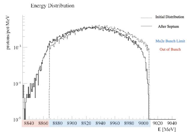
Figure 2: Energy distribution before and after passing through septum wires and applying transverse cuts. The low energy shoulder will wind up as out of time beam and integrates to 0.0168 protons/pot.
