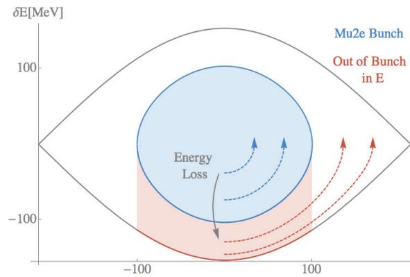
Figure 1: Longitudinal phase space bucket in the FNAL Accumulator. Energy loss will put protons in the red region, which will end up out of time after some number of turns.
