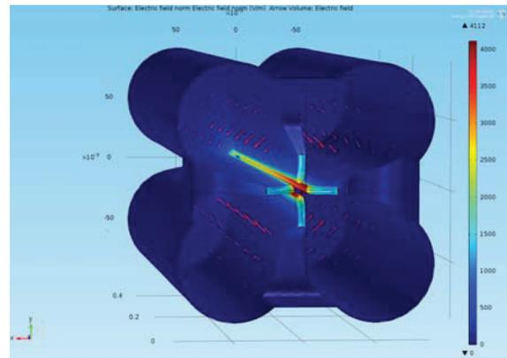
Figure 4: Abs. Electric field (V/m) on the RFQ ends for the quadrupole mode.
