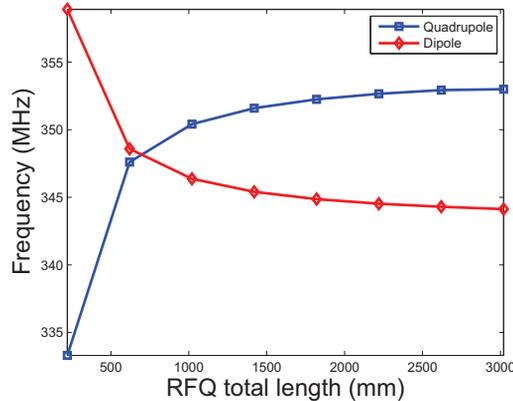
Figure 3: Variation of the RFQ resonant modes with total length.
