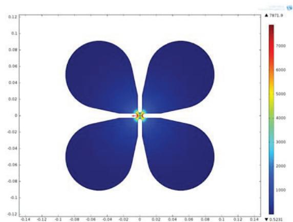
Figure 2: Abs. E field (V/m) for a 2D Dipole mode representation (XY plane at Z=0.5m). Frequency = 346 MHz.
