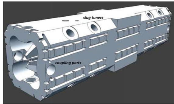
Figure 8: Layout of the ESS-Bilbao RFQ Cold-Model. Where  $L=1067.4$  mm is the total length,  $h=w=260$  mm are height and width,  $\phi_{tuner}=35$  mm is the tuner diameter and  $\phi_{coupler}=21.27$  mm is the diameter of the input power ports.
