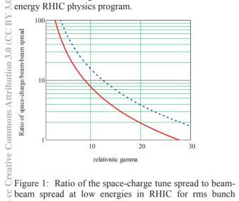
beam spread at low energies in RHIC for rms bunch length 2 m (red) and 1 m (blue, upper dash line).
