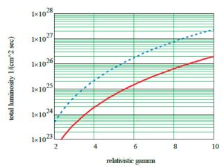
Figure 2: Projection of average total luminosity (without vertex cut) for 111 bunches of Au ions in RHIC for the space-charge tune spread of  $\Delta Q_{sc}$ =0.05: 1) blue dash upper curve - with electron cooling and long bunches (9 MHz RF); 2) red solid lower curve – without cooling and nominal bunch length (28 MHz RF).
