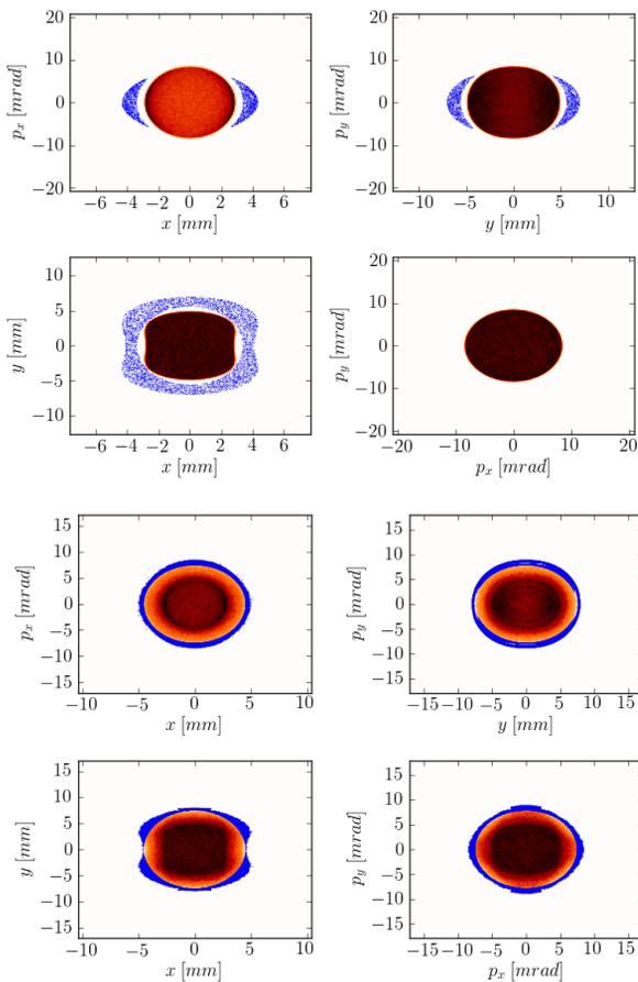
Figure 3: The initial (top) and equilibrium (bottom) beam with pre-halo in the IEL.
