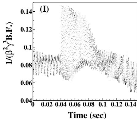
Figure 2: Calculation results of  $1/(\beta^2\gamma^3 B_f)$  when beam are accelerates by the RF voltage pattern (I).
