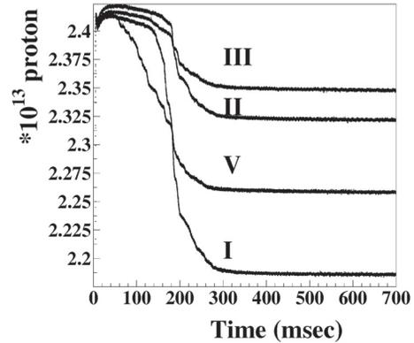
Figure 5: Beam losses measured by DCCT.
