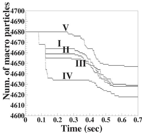
Figure 4: Beam losses for every RF voltage pattern.
