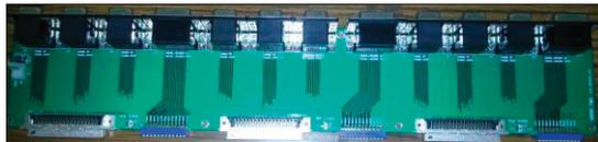
Figure 3: Eighteen motor control circuits for a cam mover system.
