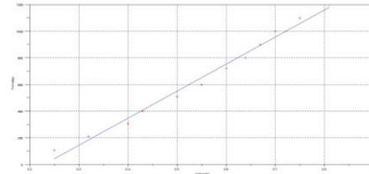
Figure 7 The relation bewteen clamping force and the the volotage.
