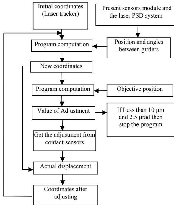
Figure 6: Illustration of testing procedure.
