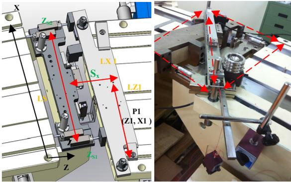
Figure 2: The local coordinate model and the linear encoder tool.
