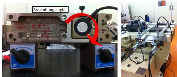
Figure 4: Assembling of the PSD sensor and the touch sensor jig.
