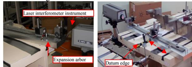
Figure 1: Laser interferometer system.
