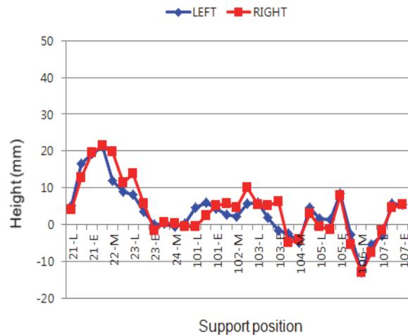
Figure 4: The floor level of the accelerator tunnel.
