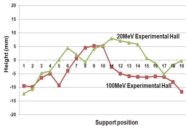
Figure 5: The floor level of the 20-MeV and 100-MeV experimental halls.
