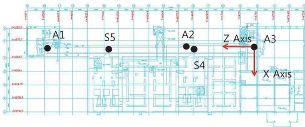
Figure 3: Coordinate system of the 100MeV proton linac. A3 is the origin and the Z axis was setup by using the coordinate of A1. The coordinates of A1 and A3 are linked with the coordinate system used for the construction.
