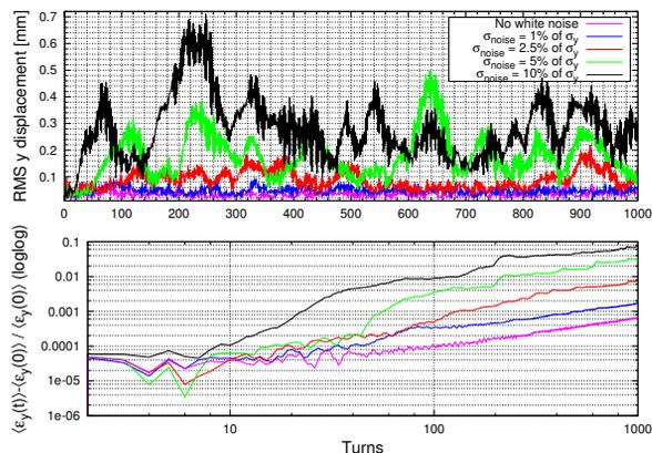
Figure 5: Rms of vertical position (top) and relative average vertical emittance growth (bottom) of the beam in the case of no white noise applied (magenta),  $\sigma_{noise} = 0.01\sigma_y$  (blue),  $\sigma_{noise} = 0.025\sigma_y$  (red),  $\sigma_{noise} = 0.05\sigma_y$  (green) and  $\sigma_{noise} = 0.1\sigma_y$  (black).
