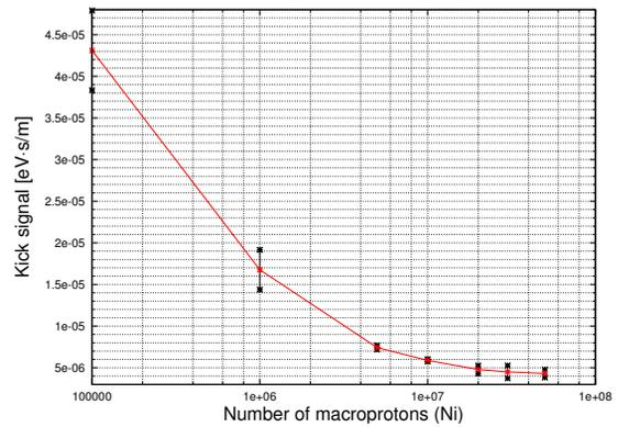
Figure 2: Minimum kicker signal required to stabilize the beam (i.e. for the vertical emittance to grow less than 0.1% over 1000 turns) as a function of  $N_i$ . The black vertical bars correspond to the error intervals, the amplitude of each interval is related to the number of simulations performed for each  $N_i$  value.
