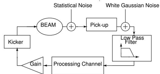
Figure 1: Complete feedback loop.
