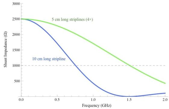
Figure 1: Shunt impedance for a single 10 cm long stripline kicker (blue) and for a set of four 5 cm long striplines (green).
