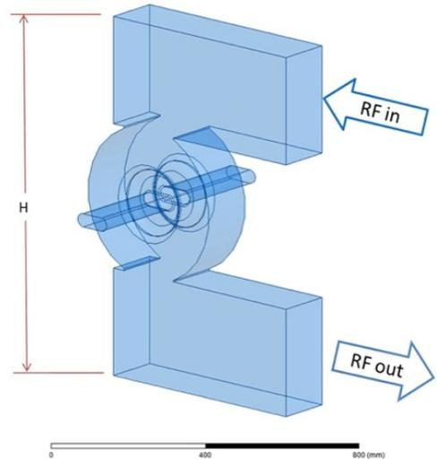
Figure 4: Model of the transverse feedback damped cavity.
