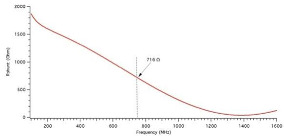
Figure 2: 10 cm stripline simulated shunt impedance (two-wire virtual measurement).
