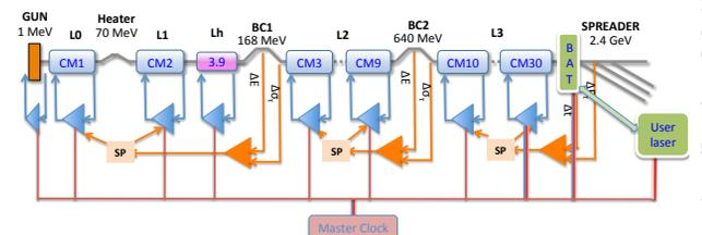
Figure 1: Layout of the NGLS with nested layers of feedback.
