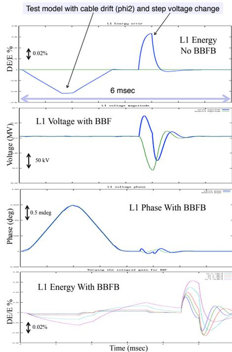
Figure 5: Initial results from the model for a single linac/bunch compressor module. a) Energy drift from RF cable drift (phi2) and a step voltage change. b) Effect of beam-based FB on voltage set point. c) effect of beam-based FB on phase set point. d) Energy drift with RF and beam-based FB at different gains.
