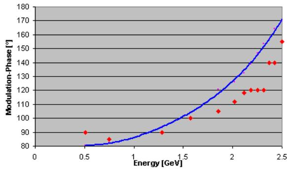
Figure 6: Behaviour of phase during ramping of energy.
