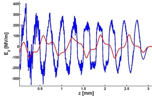
Figure 2: Computed wakefield (snapshot of the axial electric field) in a 300 GHz nonlinear dielectric structure,  $\varepsilon(E=0)=225$ ,  $a=50 \mu\text{m}$ ,  $b=61 \mu\text{m}$ , with beam parameters  $\sigma_z=50 \mu\text{m}$ . Red:  $Q=0.003 \text{ nC}$  (scaled to  $0.3 \text{ nC}$ ); Blue:  $Q=0.3 \text{ nC}$ . The center of the beam is at approximately  $2.9 \text{ mm}$ .
