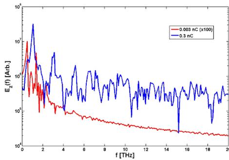
Figure 3: Spectra of the wakefields from Fig. 2. The effects of nonlinearity are apparent from the frequency upshift of the fundamental mode and the increased high frequency spectral content in the high charge data.
