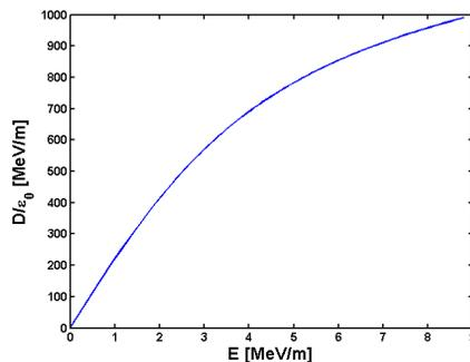
Figure 1: Approximate constitutive relation based on dynamic tunability measurements for BST(M).
