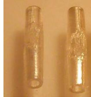
Figure 2: Single crystal diamond structures laser machined from a CVD single crystal. (ID=400, OD=700 microns)
