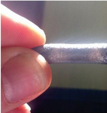
Figure 1: Diamond cylindrical waveguide fabricated from CVD polycrystalline optical quality diamond.
