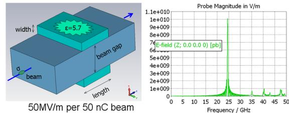
Figure 3: Left: geometry of the diamond resonator: length = 4mm, width = 1.2mm, beam gap = 4mm and overall width = 8mm. Right: spectrum of the wakefield (simulation).
