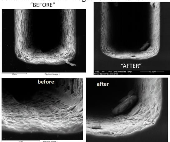
Figure 5: SEM measurement of the groove: right – before, left – after the test; lint is visible. Top: edge of the groove, Bottom: zoom on the surface.
