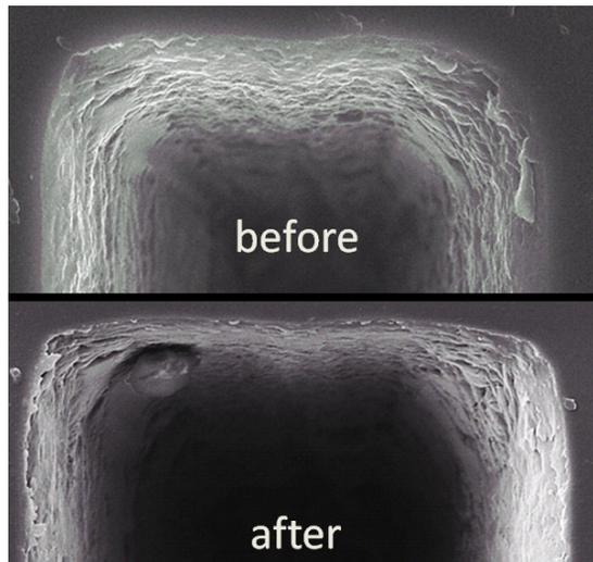
Figure 4: SEM measurement of another location along the groove: top – before, bottom – after.
