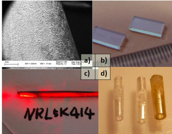
Figure 2: a) SEM image of the cylindrical diamond surface; b) single crystal CVD diamond plates for the breakdown experiment. Two collinear laser cut grooves are visible on the left piece; c) long (>1”) diamond tube, transparent to light; d) tubes laser cut from single crystal CVD diamonds (~400 microns inner diameter).
