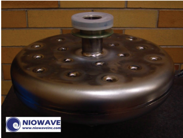
Figure 2: Photograph of the 2.1 GHz PBG cell (courtesy to Niowave, Inc.).
