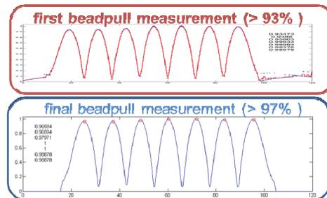
Figure 3: Bead-pulling RF measurement of first linac tank, showing good field balance across the cells.
