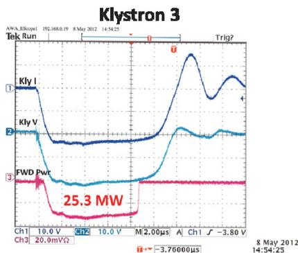
Figure 2: New Thales klystron: current, voltage and output power.
