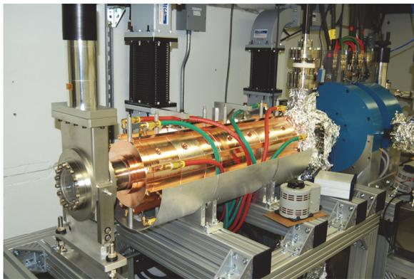
Figure 1: The new AWA RF gun (between the blue solenoids). Also shown is the first one of the six new linac tanks.
