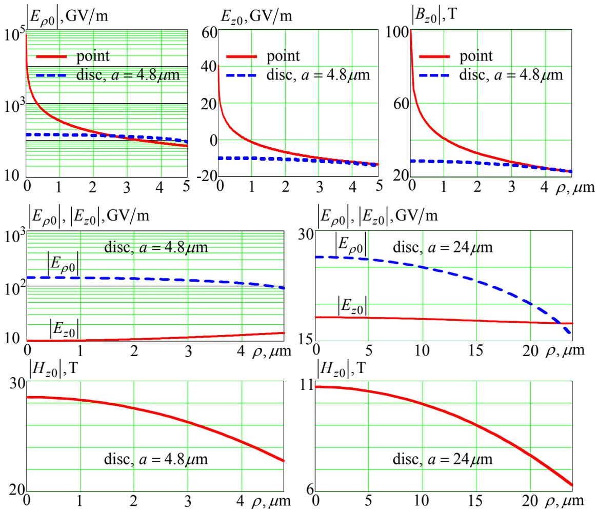
Figure 3. Magnitudes of the longitudinal and orthogonal electric field and longitudinal magnetic field versus  $\rho$ . Calculation parameters coincide with those of Fig. 2.
