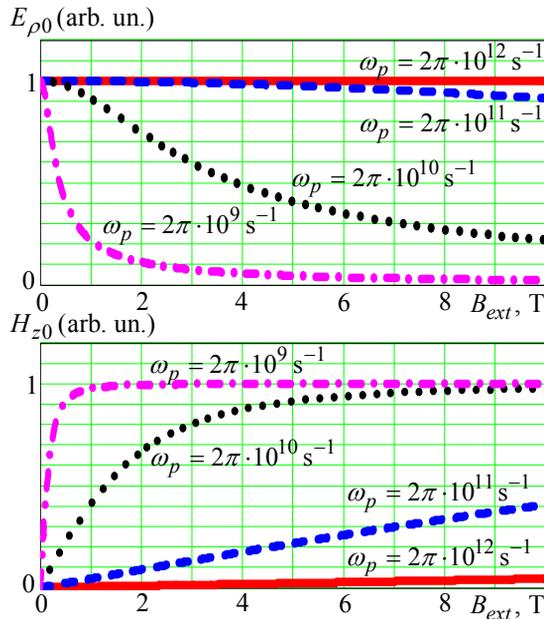
Figure 1. Magnitudes of orthogonal electric and longitudinal magnetic fields versus  $B_{ext}$ .
