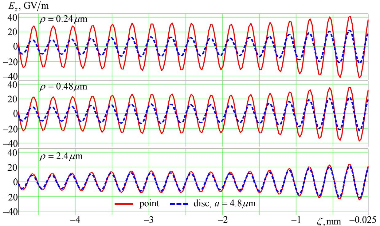
Figure 2. Longitudinal (accelerating) electric field  $E_z$  versus  $\zeta$  for different offsets  $\rho$  from the motion line. Calculation parameters are:  $\omega_p = 2\pi \cdot 10^{12} \text{ s}^{-1}$ ,  $\omega_h = 0.5\omega_p$  ( $B_{ext} = 18 \text{ T}$ ),  $\beta = 0.999$ ,  $q = -\ln C$ .
