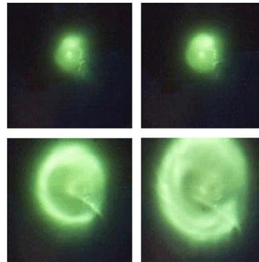
Figure 7: The optical diagnostics of compensation electrons confined in  $He^+$  ( $W=14keV$ ,  $I=2.3mA$ ) beam and solenoidal magnetic field.
