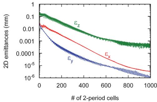
Figure 2: Horizontal  $\epsilon_x$ , vertical  $\epsilon_y$ , and longitudinal  $\epsilon_z$  emittances along the cooling channel plotted vs. the number of 2-period cells (equal to the number of passed absorbers).
