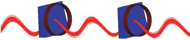
Figure 5: Muon tracks in a 0.2 m period twin helix.
