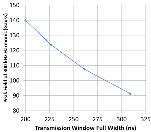
Figure 4: Required amplitude of the fundamental harmonic as a function of the transmission window, assuming a normalized admittance of 50 \pi -mm-mr.
