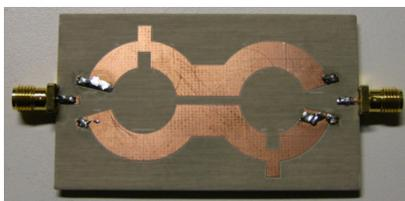
Figure 4: The back-to-back transmission loss setup of the proposed planar balun
