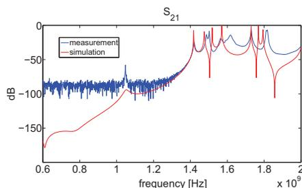
Figure 6: (color) Comparison between the simulated and measured transmission versus frequency for the spin-flip cavity.
