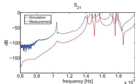
Figure 4: (color) Comparison between the simulated and measured transmission for the spin-flip cavity.
