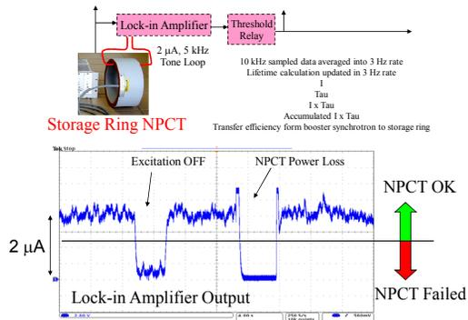
Figure 2: DCCT self-diagnostic system.
