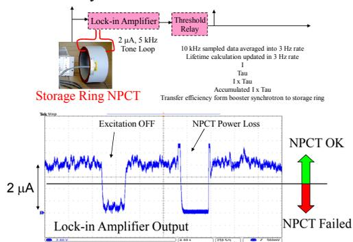
Figure 2: DCCT self-diagnostic system.
