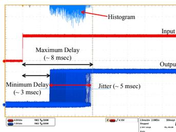
Figure 5: Slow MPS response time measurement.
