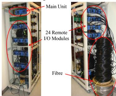
Figure 4: Full scale test bed for PLC based slow MPS.
