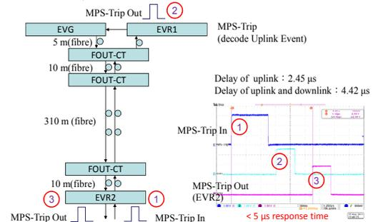
Figure 6: Fast MPS response time measurement.
