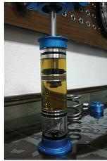
Figure 1: A schematic configuration of the hybrid damper.
