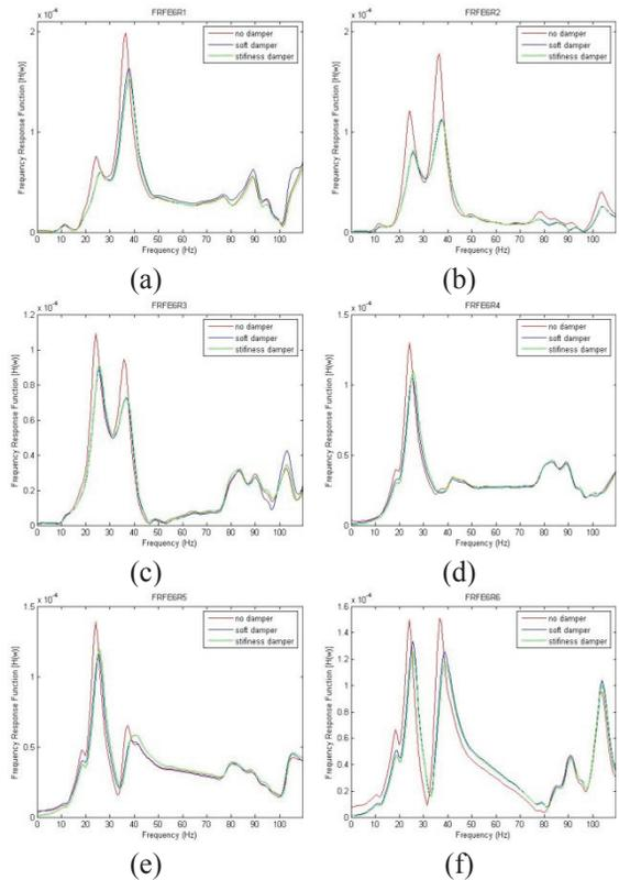
Figure 6: Typical frequency response function of acceleration data of a girder (G1) subjected to impulse excitation.
