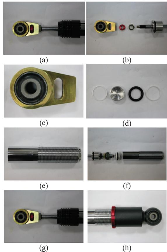
Figure 2: Components of a hybrid damper.
