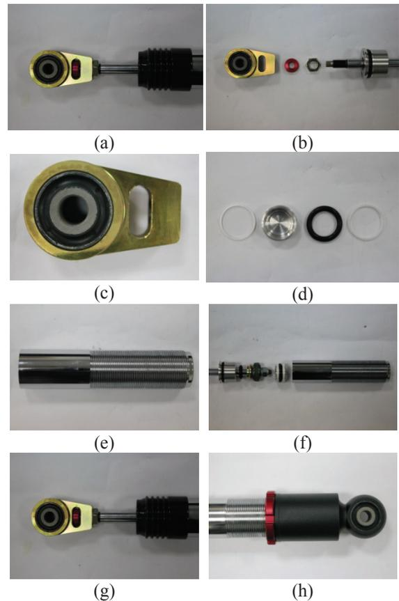
Figure 2: Components of a hybrid damper.
