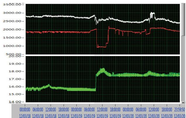
Figure 2: Supplied air temperature from AHU and power consumption histories before and after raising the air temperature setting.
