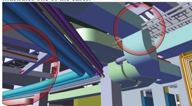
Figure 2: Interferences among pipes, cable trays and wind ducts.
