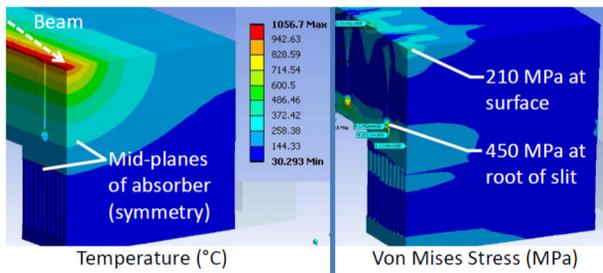
Figure 3: Simulated temperature and stress contours.
