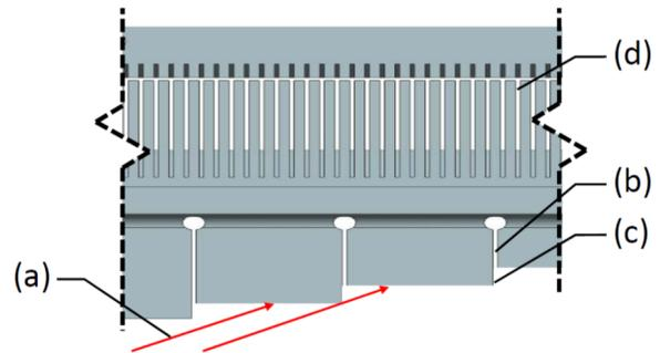
Figure 2: Side view of absorber showing (a) beam incident on surface, (b) axial stress relief slits, (c) shadowing step increment (magnitude exaggerated), (d) 300 $\mu$ m wide by 1mm pitch water cooling channels. Horizontal scale exaggerated.
