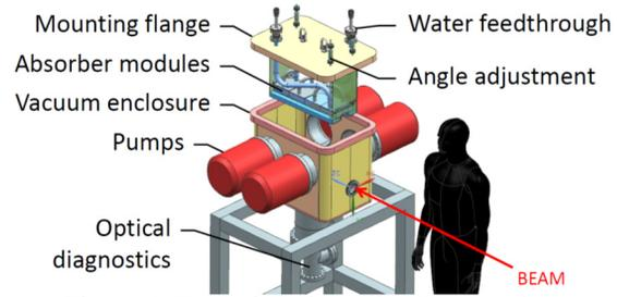
Figure 5: Exploded view of PXIE absorber.
