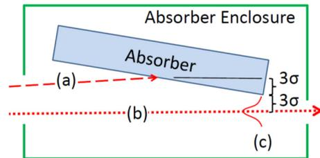
Figure 1: Schematic representation of the absorber showing (a) chopped beam, (b) passed beam, (c) beam profile and 6σ transverse shift between the centers of the chopped and passed beams.
