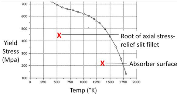
Figure 4: Stress/Temperature Conditions. Xs represent peak temperature (surface) and peak stress (slit) locations as compared to the TZM yield curve from [8].
