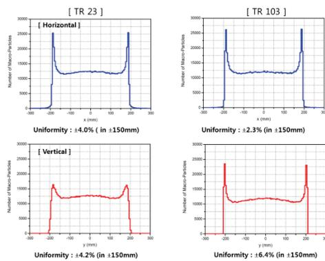
Figure 4: Transverse beam distribution at the beam window in the target room.
