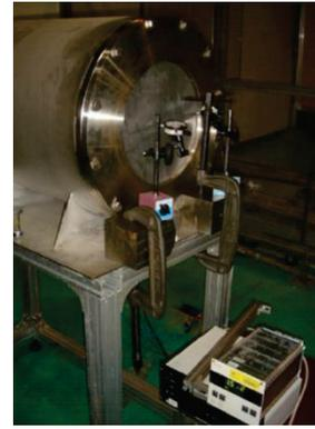
Figure 5: The fabricated AlBeMat beam window
