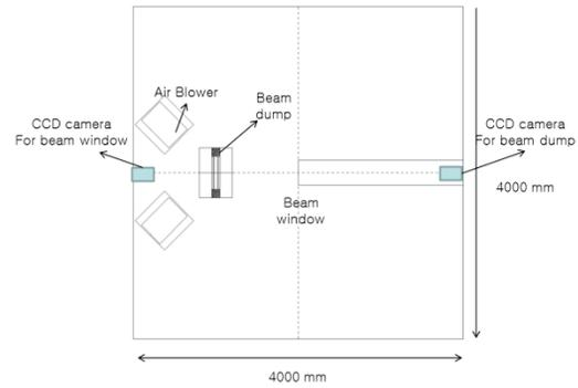
Figure 8: General arrangement of the target room.
