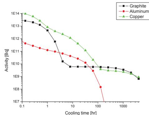
Figure 6: The residual radioactivity of the various materials.
