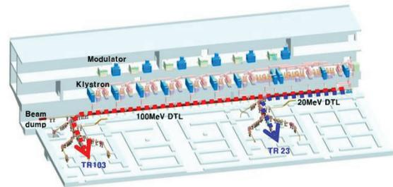
Figure 1: Layout of 100 MeV proton linac.
