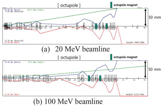
Figure 3: The transport calculation in the 20 MeV and 100 MeV proton beamlines.
