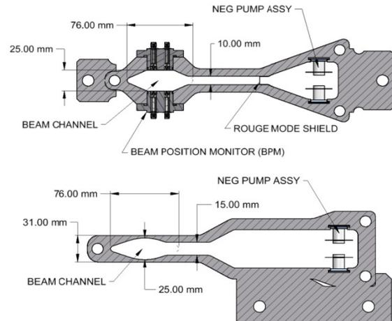
Figure 2: Extruded multipole (top) and dipole chamber cross sections
