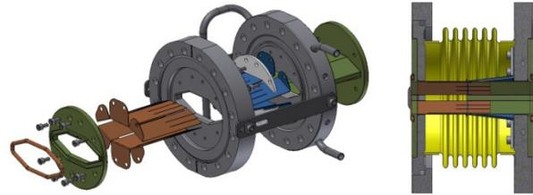
Figure 6: Exploded view of RF bellows (left) with convolutions removed and side view of completed unit
