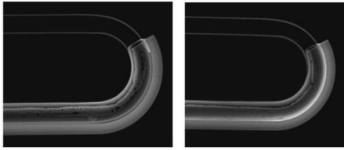
Figure 5: X-ray imaging showing incomplete braze flow (left) and complete braze flow (right)
