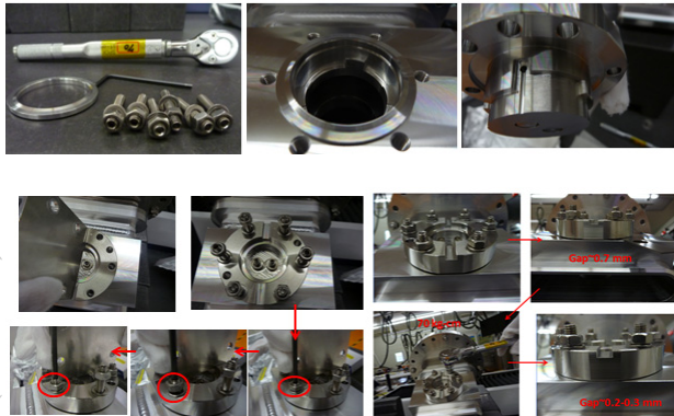
Figure 4: Pictures describing steps for sealing with a diamond-edge gasket.
