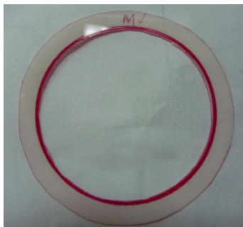
Figure 10: distribution of load on the peak of the diamond-edge gasket.
