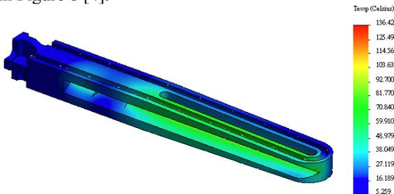
Figure 8: Thermal analysis of a crotch absorber
