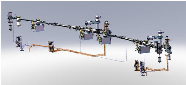
Figure 9: 3D drawing of a cooling system in one bending cell.
