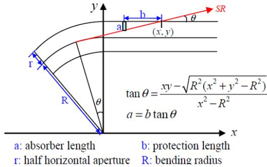
Figure 3: Sketch of synchrotron light incident on a straight section.
