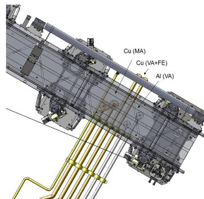
Figure 7: Manifolds under a girder.
