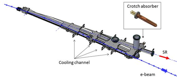
Figure 6: Layout of a B1 bending chamber.
