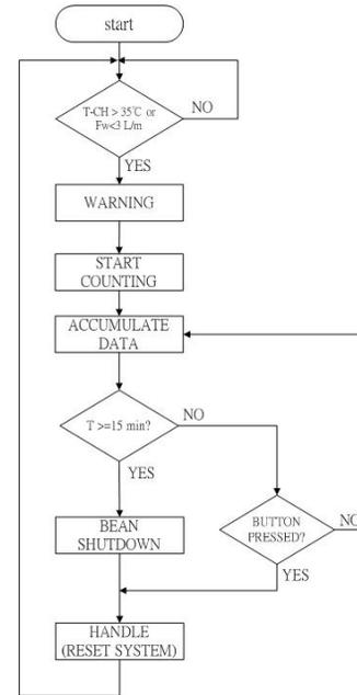
Figure 10: Logic flow chart of the temperature-monitoring system in Taiwan Light Source (TLS).
