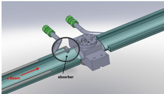
Figure 4: 3D schematic drawing of absorber in front of BPM block.
