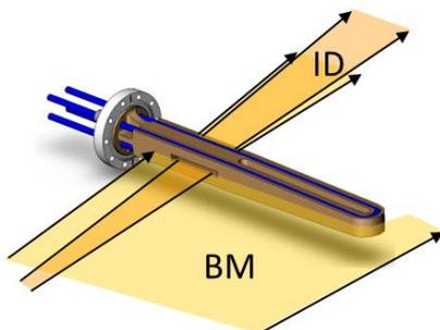
Figure 5: 3D schematic drawing of a crotch absorber.
