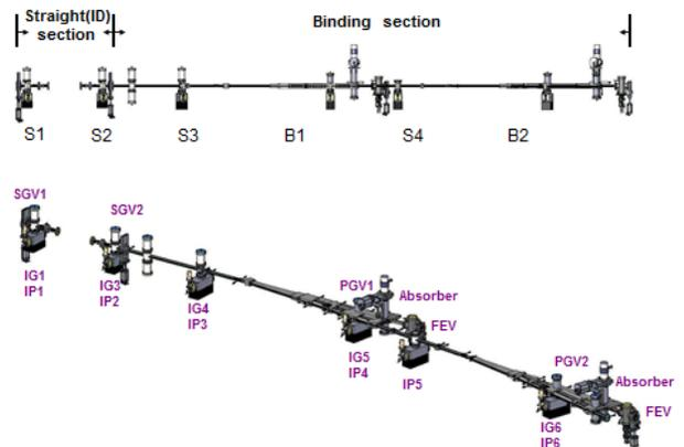
Figure 2: Layout of a typical vacuum system for one unit cell.
