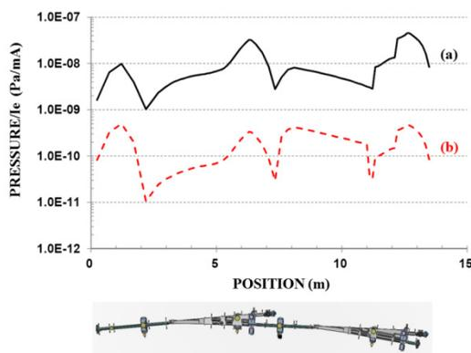
Figure 6: Curves of calculated distributed pressure per beam current, PRESSURE/Ie, for the unit-cell vacuum system at beam dose (a) 1 A h and (b) 100 A h.
