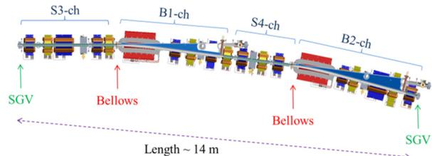
Figure 1: Schematic drawing of the transection profile for a typical 14 m arc-cell vacuum system.
