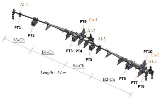
Figure 5: Layout of arc-cell vacuum system. PT1 ~ PT10 represent the ten pumping ports. Locations of four aluminium absorbers, Al-1 ~ Al-4, and two copper crotch absorbers, Cu-1 and Cu-2, inside the vacuum chambers are indicated.
