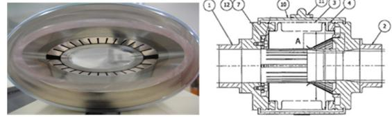
Figure 3: Photograph of the rf fingers and schematic drawing for the bellows.
