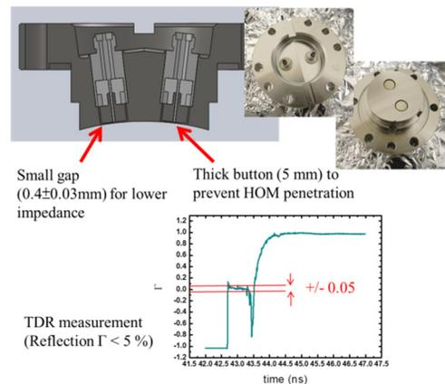
Figure 4: Drawing and photograph for the BPM-flanges, and the reflection coefficient measured by TDR.
