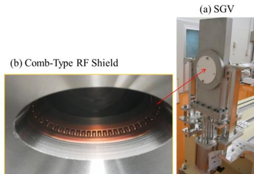
Figure 2: Photographs of the (a) sector gate valve (SGV) and (b) comb-type rf shield.
